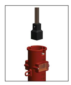
Remove the Body (10) from the Standpipe (8) by loosening the upper two Hex Bolts (7) and Hex Nuts (6). Then remove the Standpipe (8) from the Base Flange (5) by loosening the lower two Hex Bolts (7) and Hex Nuts (6).
