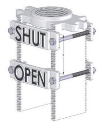
If the Non-rising Stem Gate Valve is opened right: Move the two Shut Targets (16) to the very top of the Target Carrier Nut (12). Locate the two Open Targets (16) according to the Non-rising Stem Gate Valve stem size target distance below ("X").
